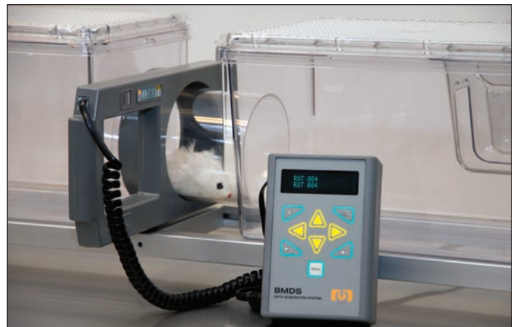
Ring Reader with tunnel for connection of cages. Can be used in behavior studies.
