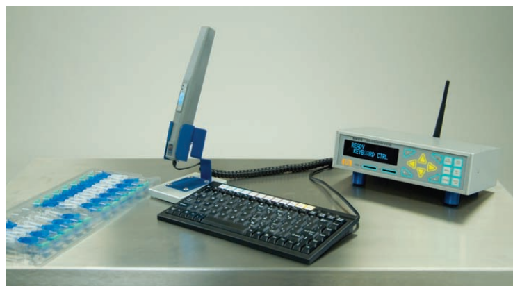
Programming station with SP 6005 and optional keyboard, shown here with DAS-6001 Console System
